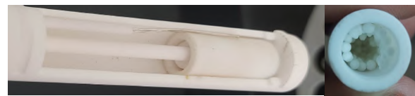
Figure 1 Pebble bed arrangement and sintered pebbles after the experiment
